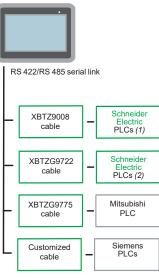
Examples of connection to RS-422/RS-485 serial port (3)
